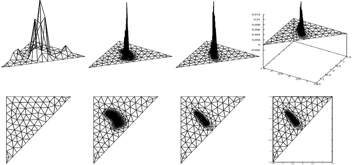
Fig. 2. Measure  $\mu(\mathbb{P}_k^{(\ell)}, w_1^\ell, \dots, w_k^\ell)$  and the supporting (fictitious) triangulation  $\mathbb{P}_k^{(\ell)}$  during adaptive refinement/coarsening procedure iterations  $\ell = 1, 2, 4$  and  $7$ .
