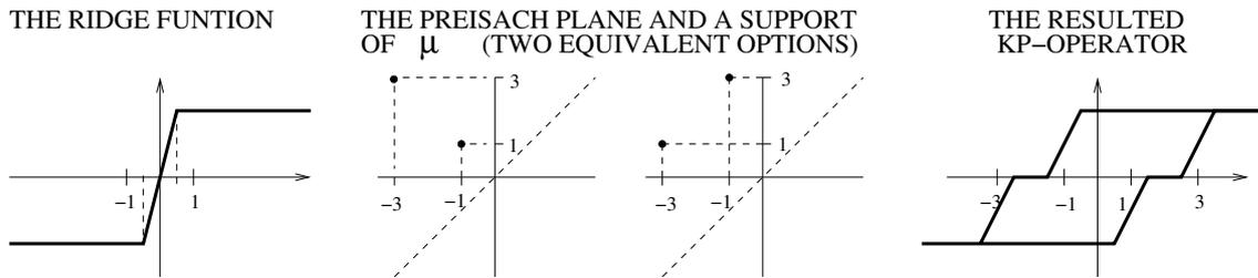
Fig. 4. Example on non-uniqueness: both  $\mu = \frac{1}{2}\delta_{(-h_1, h_1)} + \frac{1}{2}\delta_{(-h_2, h_2)}$  and  $\mu = \frac{1}{2}\delta_{(-h_2, h_1)} + \frac{1}{2}\delta_{(-h_1, h_2)}$  are solutions if only the parent loop is traced.
