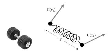
We describe polymer chains as two beads connected by a spring, q is the vector connecting the beads.
