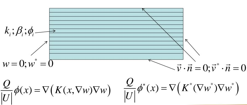
$$(k^*)^{-1} = \sum_{i} k_i^{-1} \frac{h_i}{H} \left(\frac{\phi_i}{\phi^*}\right)^2; \frac{\beta^*}{k^*} = \sum_{i} \frac{\beta_i h_i}{k_i H} \left(\frac{\phi_i}{\phi^*}\right)^3$$
